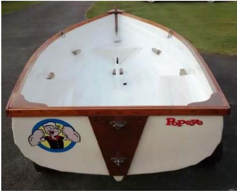
The transom rudder and outboard mount done and new wooden blocks being made in DT class at school with the help of Mr. Kettlewell.
