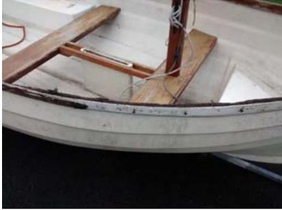
The gunwales and all the timber trim were in a very poor state and needed replacing.
