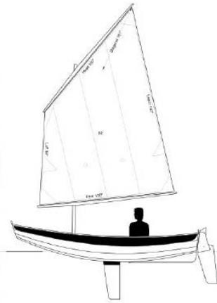
I re-rigged Popeye with a balanced lug, with the yard mount 1/3rd along its length and the tack mounted forward of the mast so there is almost an even length of sail from top to bottom ahead of the mast. The sail area in front of the mast helps balance the sail area aft, thus the name, so sheeting loads are lighter.
